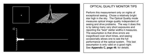
When the graphic information is on the video screen you can toggle on the 3 dimensional graph of the star profile by hitting the **Value** button again. Displaying the 3D graph will slow the update rate. As the graph is updating, the alphanumeric display provides the quantitative data:
