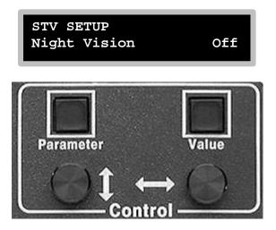
You would then press the **Value** button under the word "Off" or turn the rotary knob directly under the **Value** button until the display reads:
