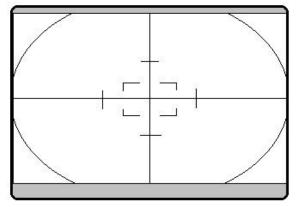
Normal + Full: The central 640x400 pixels are binned 2x2 and displayed to fill the video screen horizontally. Good balance of sensitivity and resolution. Good mode for galaxies.
