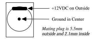
**Caution:** The STV will draw approximately 2 amps of current, which can drain a car batter to low levels over the course of an evening. It may be wise to use a separate battery to run the STV if you intend to image for any significant length of time, particularly if you are also running an external monitor and/or telescope mount from the same battery. Deep discharge marine batteries are recommended.
