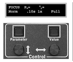
Focusing Tips: Note the location of the words "Norm" and "Full" on the display and in relation to the buttons below the display. Pressing the **Parameter** button will toggle the Zoom mode: Norm, Zoom, Wide. Pressing the **Value** button will toggle the image size on the video screen: Full or Partial. These functions may be invoked in any combination to select, for instance, a video image that is Zoom and
