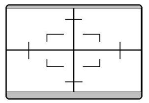
Zoom + Full: The central 320x200 pixels are displayed unbinned (1x1) to fill the video screen horizontally. This mode has the lowest sensitivity and highest resolution. Best for moon and planets.
