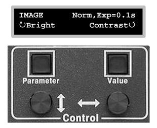
In Image Capture Mode (unlike focus mode) the rotary knobs do not change the exposure time of the image. Rather, the exposure time is selected in the Image Setup Menu and the rotary knobs control the brightness and contrast of the image. The display shows small circular arrows prompting you to adjust the Brightness and Contrast to suit your monitor. Pressing the Parameter button in Image Mode will toggle through the zoom levels. Pressing the Value button has no effect in Image Mode.
