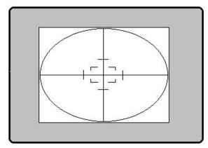
Wide + Full: The entire 656x480 pixels are binned 3x3 and displayed in a window in the center of the video screen. This gives the widest field of view and is the most sensitive mode. Best for imaging large dim objects
