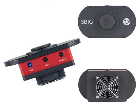
The STC-7 scientific CMOS camera represents a major improvement over CCD technology. Compared with previous CCD models, the STC-7 features higher sensitivity (78% QE versus 56%), significantly lower read noise (2.5 e- versus 9.3 e-), and 20X faster readout. While a single exposure can equal CCD dynamic range, the combination of fast readout and very low read noise allows for in-camera stacking using SBIG's StackPro™ to produce a greater dynamic range than previously possible.
