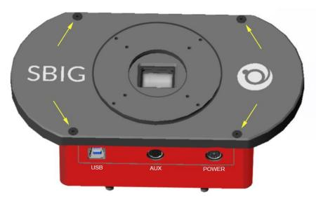
3. Remove the eight indicated screws securing the filter retainer using the supplied 1/20" Allen key and remove the retainer from the carousel. (Filter slots are round – the rectangular mask works as a baffle for the sensor.)
