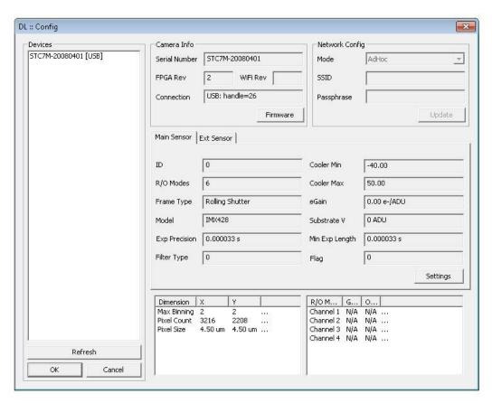
This form allows you to check camera parameters and also to perform firmware updates and additional camera configuration.
