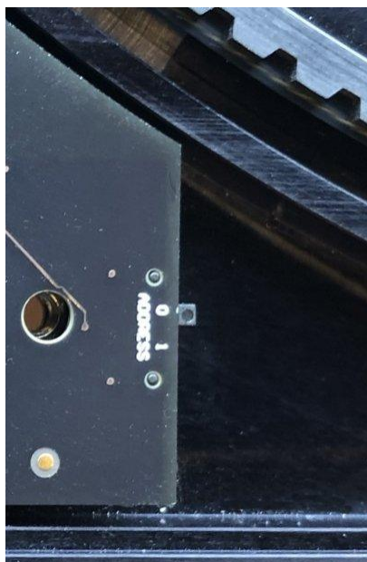
Address Switch Up (0) for Filter Wheel 1 Down (1) for Filter Wheel 2
